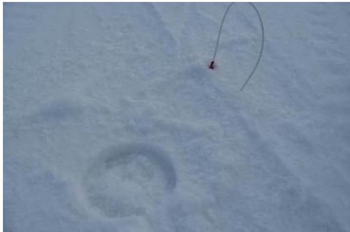
Oil sample (400 mL) drilled into the ice and left for a week
