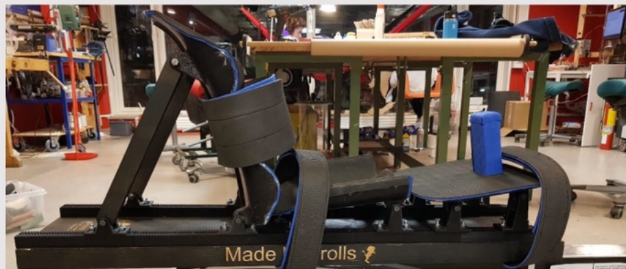
Figure 5 - 3D printed PR1 seating assembly used in the world indoor rowing championship.
